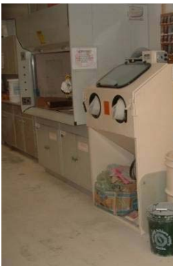
FUME HOOD, SAND BLAST ABRASION CENTER
