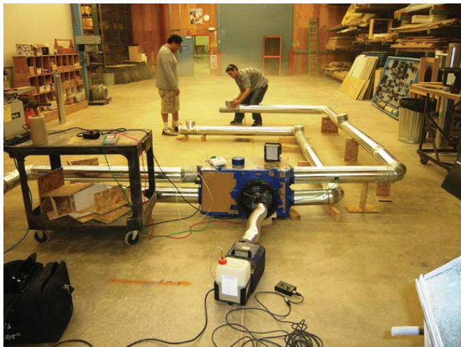
Photo 3.36 TEC Construction Technology - Blower Door Testing
